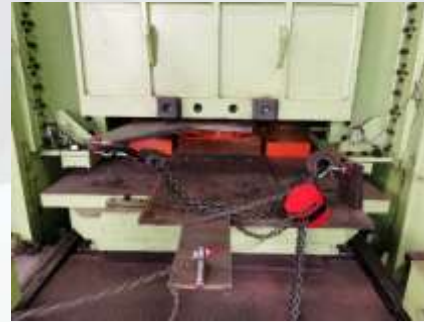
10T手拉葫芦装载于牵引反力架
